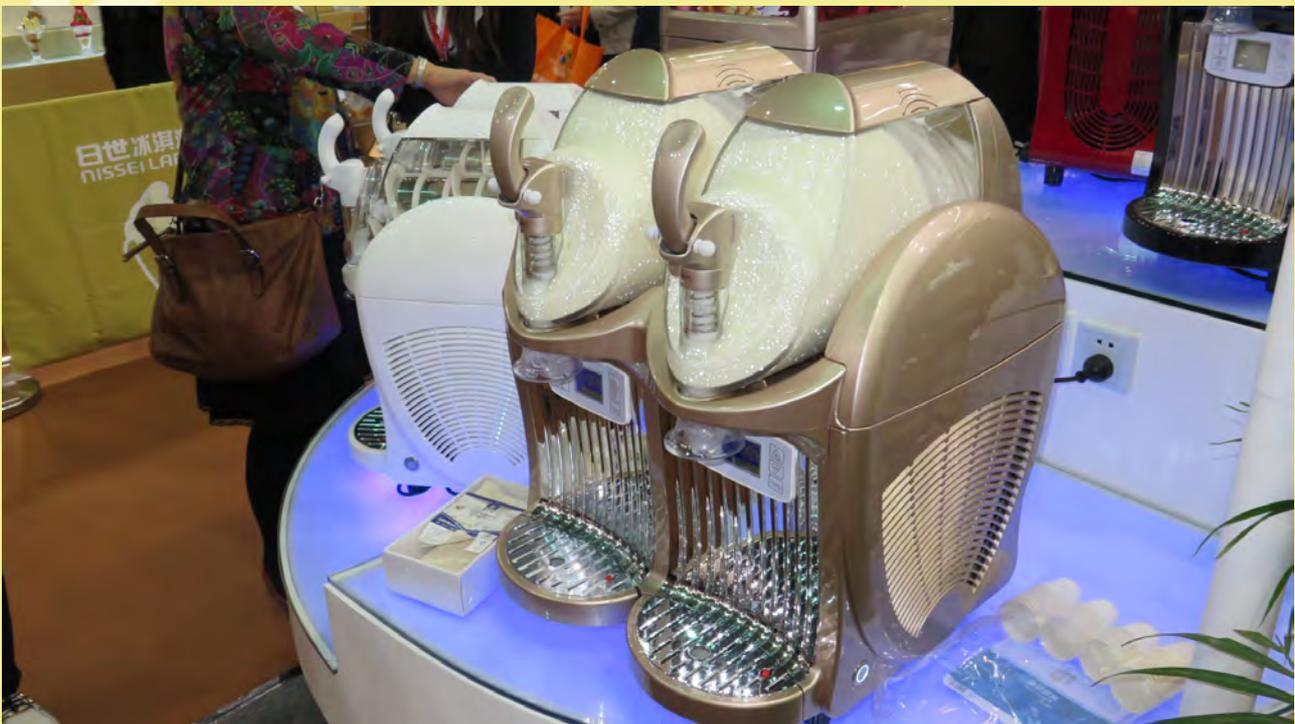
**Soft Serve Slush:** A less expensive way to make soft serve is with a modified slush machine. “Slush” also called “granita” is a semi-frozen drink usually made with a countertop machine, which consists of a freezing compressor and a screw-type rotating “dasher” or churning blade rotating inside a clear plastic tank. “Slush” is extruded at about -3C. Soft serve slush is extruded at about -6C. This may seem like a small difference but it’s not!
